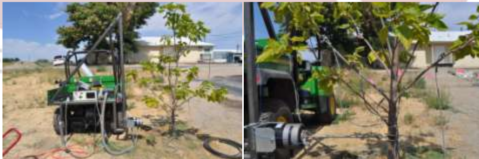
Figure 5. Frequency response test on a central leader tree
